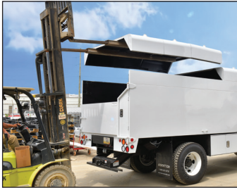
Lift rear sections off
