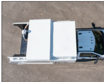
Manually slide roof sections forward
